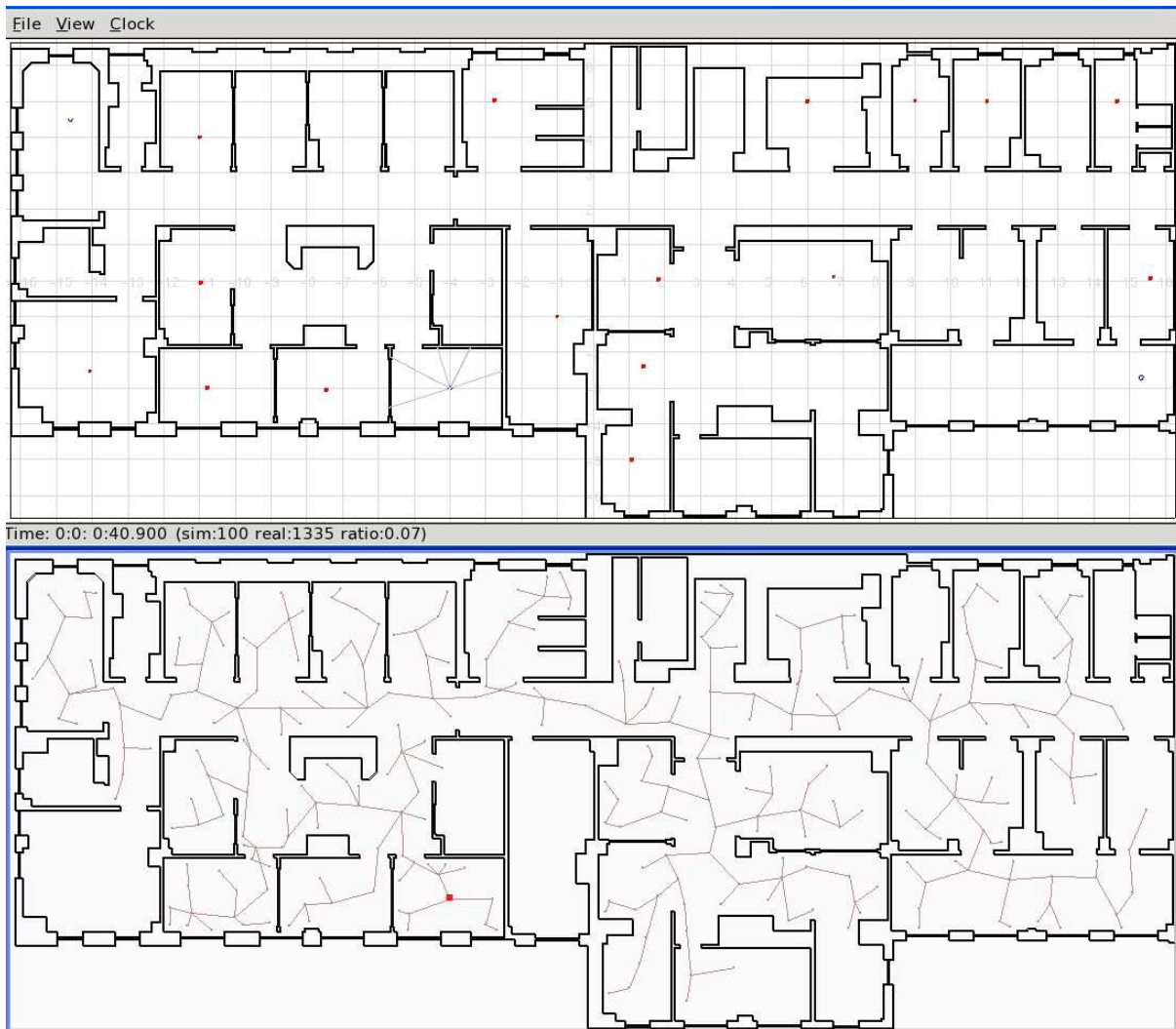
Figure 1: The hospital environment. The top part of the figure shows the Stage simulation, with the locations of the tasks and of the robots. (The active robot has its range sensor traces shown). The lower part shows the paths generated by the RRT algorithm, with the location of the active robot on the paths indicated by a square. This is one of the single robot experimental runs, where only one robot is active.
